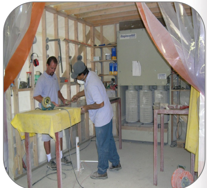
RECOMMENDED DRY ROOM BOOTH ENCLOSURE SHOWING NEGATIVE PRESSURE CONCEPT AND AIR FLOW PATTERNS
